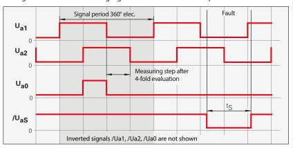
The distance between two successive edges of the incremental signals U<sub>a1</sub> and U<sub>a2</sub> through 1-fold, 2-fold or 4-fold evaluation is one measuring
